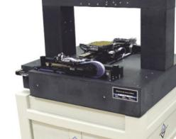
Multi-axis air-bearing with granite bridge and a machine base
